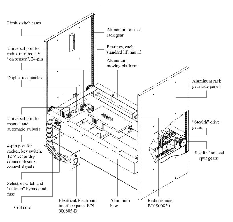
Unit is shown with radio remote controller 900820 and electrical/electronic interface panel 900805-D, both of which are accessories.
