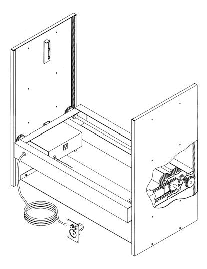
The Inca lift is a motorized rack and pinion lifting machine providing the least costly solution to concealing your TV in a cabinet. This lift has a standard, fit all size, to accommodate the most commonly found televisions. The robust lifting capacity of 200 lbs allows this machine to support a wide range of applications.
