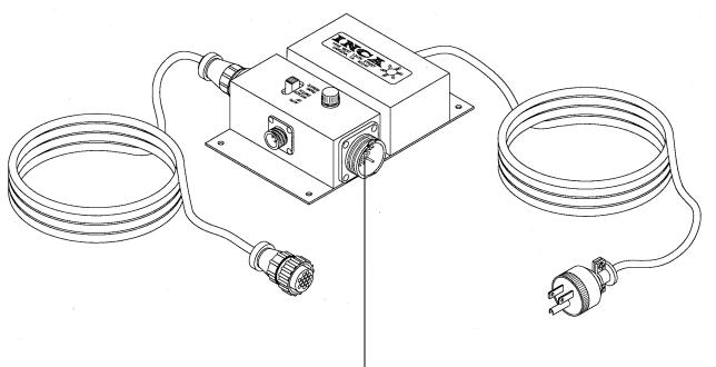
External universal J-box to attach the controllers to the lift and swivel
