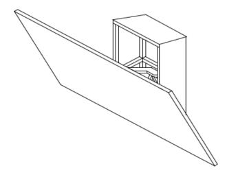
This tilting module can be used with or without a fabricated enclosure around the TV.
