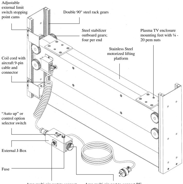
Amp multi-pin port to connect rocker switch, 12 VDC external control or dry contact touch screen controller Amp multi-pin port to connect RF, single or multi-channel (auto-swivel) controllers or infrared TV "on" sensor
